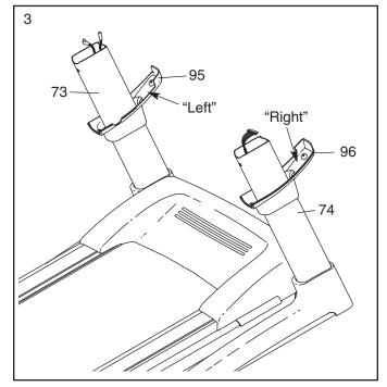
4. With the help of a second person, hold the console assembly near the Uprights (73, 74).
